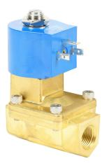
GC Valves potable water solenoid valve, 2-port (2-way), 2-position, N.C., lead-free brass body, EPDM rubber seal(s), 3/8in female NPT inlet(s), 3/8in female NPT outlet(s), Cv=4.3, 24 VDC operating voltage, 9W, NSF/ANSI 61.
