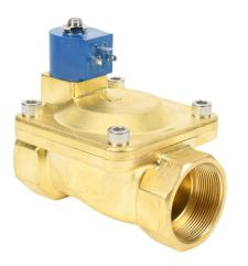
GC Valves potable water solenoid valve, 2-port (2-way), 2-position, N.C., lead-free brass body, EPDM rubber seal(s), 2in female NPT inlet(s), 2in female NPT outlet(s), Cv=48, 120 VAC operating voltage, 8W, NSF/ANSI 61.
