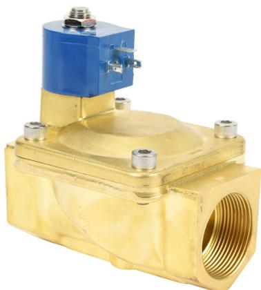
GC Valves potable water solenoid valve, 2-port (2-way), 2-position, N.C., lead-free brass body, EPDM rubber seal(s), 1-1/2in female NPT inlet(s), 1-1/2in female NPT outlet(s), Cv=30, 120 VAC operating voltage, 8W, NSF/ANSI 61.
