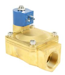
GC Valves potable water solenoid valve, 2-port (2-way), 2-position, N.C., lead-free brass body, EPDM rubber seal(s), 1-1/4in female NPT inlet(s), 1-1/4in female NPT outlet(s), Cv=22, 120 VAC operating voltage, 8W, NSF/ANSI 61.
