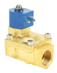
GC Valves potable water solenoid valve, 2-port (2-way), 2-position, N.C., lead-free brass body, EPDM rubber seal(s), 1in female NPT inlet(s), 1in female NPT outlet(s), Cv=13, 120 VAC operating voltage, 8W, NSF/ANSI 61.
