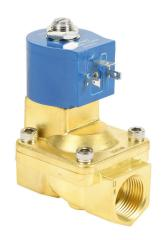
GC Valves potable water solenoid valve, 2-port (2-way), 2-position, N.C., lead-free brass body, EPDM rubber seal(s), 3/4in female NPT inlet(s), 3/4in female NPT outlet(s), Cv=6.7, 120 VAC operating voltage, 8W, NSF/ANSI 61.
