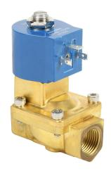
GC Valves potable water solenoid valve, 2-port (2-way), 2-position, N.C., lead-free brass body, EPDM rubber seal(s), 1/2in female NPT inlet(s), 1/2in female NPT outlet(s), Cv=4.3, 120 VAC operating voltage, 8W, NSF/ANSI 61.
