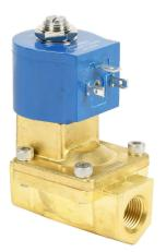
GC Valves potable water solenoid valve, 2-port (2-way), 2-position, N.C., lead-free brass body, EPDM rubber seal(s), 3/8in female NPT inlet(s), 3/8in female NPT outlet(s), Cv=4.3, 120 VAC operating voltage, 8W, NSF/ANSI 61.
