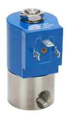
GC Valves potable water solenoid valve, 2-port (2-way), 2-position, N.C., 303 stainless steel body, 1/4in female NPT inlet(s), 1/4in female NPT outlet(s), Cv=0.85, 24 VAC operating voltage, 10W, NSF/ANSI/CAN 61.
