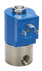
GC Valves potable water solenoid valve, 2-port (2-way), 2-position, N.C., 303 stainless steel body, 1/4in female NPT inlet(s), 1/4in female NPT outlet(s), Cv=0.36, 24 VAC operating voltage, 10W, NSF/ANSI/CAN 61.
