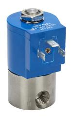
GC Valves potable water solenoid valve, 2-port (2-way), 2-position, N.C., 303 stainless steel body, 1/4in female NPT inlet(s), 1/4in female NPT outlet(s), Cv=0.21, 24 VAC operating voltage, 10W, NSF/ANSI/CAN 61.
