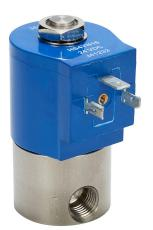
GC Valves potable water solenoid valve, 2-port (2-way), 2-position, N.C., 303 stainless steel body, 1/4in female NPT inlet(s), 1/4in female NPT outlet(s), Cv=0.36, 24 VDC operating voltage, 10W, NSF/ANSI/CAN 61.
