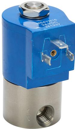
GC Valves potable water solenoid valve, 2-port (2-way), 2-position, N.C., 303 stainless steel body, 1/4in female NPT inlet(s), 1/4in female NPT outlet(s), Cv=0.21, 24 VDC operating voltage, 10W, NSF/ANSI/CAN 61.
