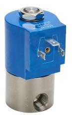
GC Valves potable water solenoid valve, 2-port (2-way), 2-position, N.C., 303 stainless steel body, 1/4in female NPT inlet(s), 1/4in female NPT outlet(s), Cv=0.21, 24 VDC operating voltage, 10W, NSF/ANSI/CAN 61.
