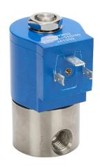
GC Valves potable water solenoid valve, 2-port (2-way), 2-position, N.C., 303 stainless steel body, 1/4in female NPT inlet(s), 1/4in female NPT outlet(s), Cv=0.85, 120/110 VAC operating voltage, 10W, NSF/ANSI/CAN 61.
