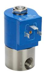
GC Valves potable water solenoid valve, 2-port (2-way), 2-position, N.C., 303 stainless steel body, 1/4in female NPT inlet(s), 1/4in female NPT outlet(s), Cv=0.36, 120/110 VAC operating voltage, 10W, NSF/ANSI/CAN 61.
