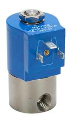
GC Valves potable water solenoid valve, 2-port (2-way), 2-position, N.C., 303 stainless steel body, 1/4in female NPT inlet(s), 1/4in female NPT outlet(s), Cv=0.21, 120/110 VAC operating voltage, 10W, NSF/ANSI/CAN 61.
