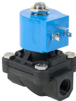
GC Valves potable water solenoid valve, 2-port (2-way), 2-position, N.C., Nylon 6 body, EPDM rubber seal(s), 3/8in female NPT inlet(s), 3/8in female NPT outlet(s), Cv=4.3, 24 VAC operating voltage, 8W, NSF/ANSI/CAN 61.
