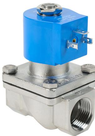
GC Valves potable water solenoid valve, 2-port (2-way), 2-position, N.C., 316 stainless steel body, 3/4in female NPT inlet(s), 3/4in female NPT outlet(s), Cv=6.7, 24 VAC operating voltage, 8W, NSF/ANSI/CAN 61.
