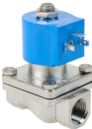
GC Valves potable water solenoid valve, 2-port (2-way), 2-position, N.C., 316 stainless steel body, EPDM rubber seal(s), 1/2in female NPT inlet(s), 1/2in female NPT outlet(s), Cv=4.3, 24 VAC operating voltage, 8W, NSF/ANSI/CAN 61.
