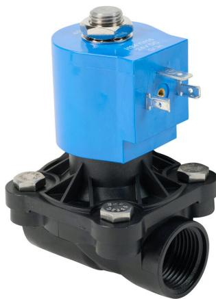
GC Valves potable water solenoid valve, 2-port (2-way), 2-position, N.C., Nylon 6 body, 3/4in female NPT inlet(s), 3/4in female NPT outlet(s), Cv=6.7, 24 VDC operating voltage, 10W, NSF/ANSI/CAN 61.
