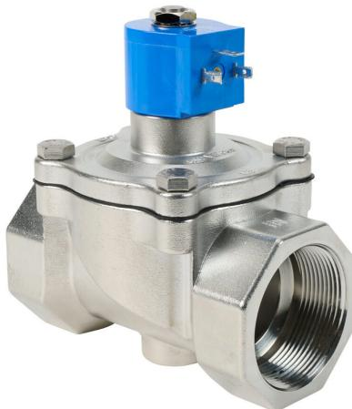
GC Valves potable water solenoid valve, 2-port (2-way), 2-position, N.C., 316 stainless steel body, EPDM rubber seal(s), 2in female NPT inlet(s), 2in female NPT outlet(s), Cv=13, 24 VDC operating voltage, 10W, NSF/ANSI/CAN 61.
