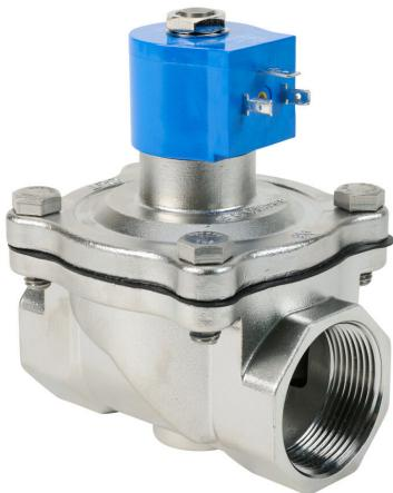
GC Valves potable water solenoid valve, 2-port (2-way), 2-position, N.C., 316 stainless steel body, EPDM rubber seal(s), 1-1/2in female NPT inlet(s), 1-1/2in female NPT outlet(s), Cv=13, 24 VDC operating voltage, 10W, NSF/ANSI/CAN 61.
