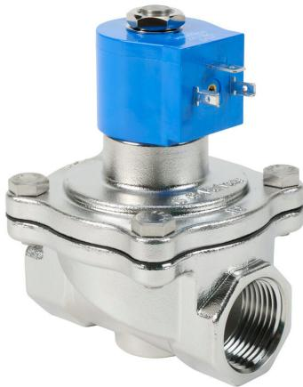
GC Valves potable water solenoid valve, 2-port (2-way), 2-position, N.C., 316 stainless steel body, 1in female NPT inlet(s), 1in female NPT outlet(s), Cv=13, 24 VDC operating voltage, 10W, NSF/ANSI/CAN 61.
