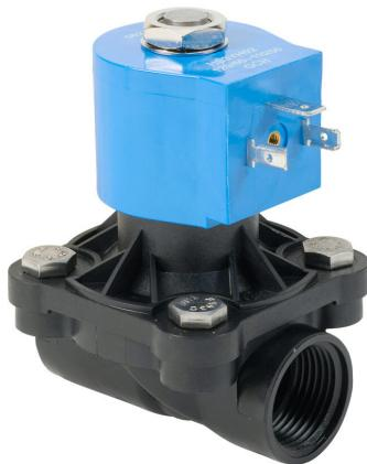
GC Valves potable water solenoid valve, 2-port (2-way), 2-position, N.C., Nylon 6 body, 3/4in female NPT inlet(s), 3/4in female NPT outlet(s), Cv=6.7, 120/110 VAC operating voltage, 8W, NSF/ANSI/CAN 61.
