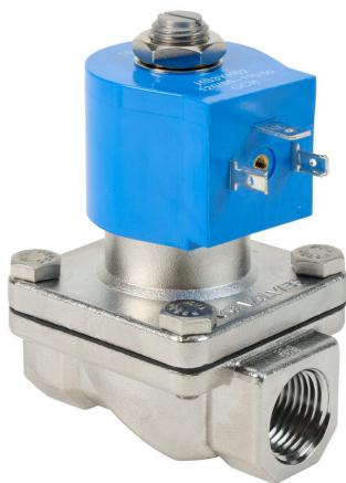
GC Valves potable water solenoid valve, 2-port (2-way), 2-position, N.C., 316 stainless steel body, EPDM rubber seal(s), 1/2in female NPT inlet(s), 1/2in female NPT outlet(s), Cv=4.3, 120/110 VAC operating voltage, 8W, NSF/ANSI/CAN 61.
