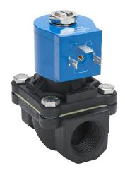
GC Valves potable water solenoid valve, 2-port (2-way), 2-position, N.C., Nylon 6 body, 3/4in female NPT inlet(s), 3/4in female NPT outlet(s), Cv=6.7, 24 VAC operating voltage, 8W.
