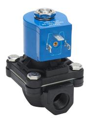
GC Valves potable water solenoid valve, 2-port (2-way), 2-position, N.C., Nylon 6 body, 3/8in female NPT inlet(s), 3/8in female NPT outlet(s), Cv=4.3, 24 VAC operating voltage, 8W.
