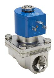
GC Valves potable water solenoid valve, 2-port (2-way), 2-position, N.C., 316 stainless steel body, 3/4in female NPT inlet(s), 3/4in female NPT outlet(s), Cv=6.7, 24 VAC operating voltage, 8W.
