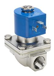
GC Valves potable water solenoid valve, 2-port (2-way), 2-position, N.C., 316 stainless steel body, 1/2in female NPT inlet(s), 1/2in female NPT outlet(s), Cv=4.3, 24 VAC operating voltage, 8W.
