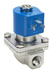
GC Valves potable water solenoid valve, 2-port (2-way), 2-position, N.C., 316 stainless steel body, 3/8in female NPT inlet(s), 3/8in female NPT outlet(s), Cv=4.3, 24 VAC operating voltage, 8W.
