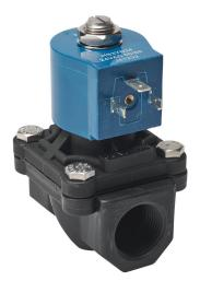
GC Valves potable water solenoid valve, 2-port (2-way), 2-position, N.C., Nylon 6 body, 3/4in female NPT inlet(s), 3/4in female NPT outlet(s), Cv=6.7, 24 VAC operating voltage, 8W, NSF/ ANSI/CAN 61.
