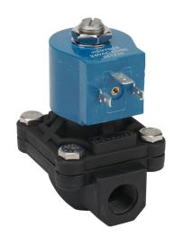
GC Valves potable water solenoid valve, 2-port (2-way), 2-position, N.C., Nylon 6 body, 3/8in female NPT inlet(s), 3/8in female NPT outlet(s), Cv=4.3, 24 VAC operating voltage, 8W, NSF/ANSI/CAN 61.
