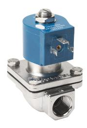
GC Valves potable water solenoid valve, 2-port (2-way), 2-position, N.C., 316 stainless steel body, 1/2in female NPT inlet(s), 1/2in female NPT outlet(s), Cv=4.3, 24 VAC operating voltage, 8W, NSF/ANSI/CAN 61.
