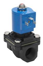
GC Valves potable water solenoid valve, 2-port (2-way), 2-position, N.C., Nylon 6 body, 3/4in female NPT inlet(s), 3/4in female NPT outlet(s), Cv=6.7, 24 VDC operating voltage, 10W.
