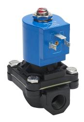
GC Valves potable water solenoid valve, 2-port (2-way), 2-position, N.C., Nylon 6 body, 3/8in female NPT inlet(s), 3/8in female NPT outlet(s), Cv=4.3, 24 VDC operating voltage, 10W.
