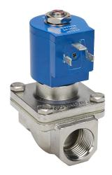
GC Valves potable water solenoid valve, 2-port (2-way), 2-position, N.C., 316 stainless steel body, 3/4in female NPT inlet(s), 3/4in female NPT outlet(s), Cv=6.7, 24 VDC operating voltage, 10W.
