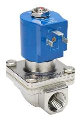
GC Valves potable water solenoid valve, 2-port (2-way), 2-position, N.C., 316 stainless steel body, 1/2in female NPT inlet(s), 1/2in female NPT outlet(s), Cv=4.3, 24 VDC operating voltage, 10W.
