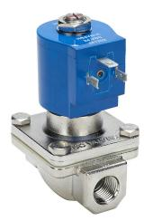
GC Valves potable water solenoid valve, 2-port (2-way), 2-position, N.C., 316 stainless steel body, 3/8in female NPT inlet(s), 3/8in female NPT outlet(s), Cv=4.3, 24 VDC operating voltage, 10W.
