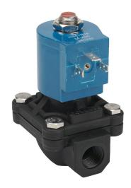
GC Valves potable water solenoid valve, 2-port (2-way), 2-position, N.C., Nylon 6 body, 3/8in female NPT inlet(s), 3/8in female NPT outlet(s), Cv=4.3, 24 VDC operating voltage, 10W, NSF/ANSI/CAN 61.
