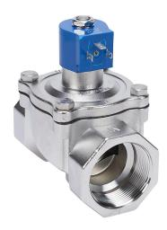
GC Valves potable water solenoid valve, 2-port (2-way), 2-position, N.C., 316 stainless steel body, 2in female NPT inlet(s), 2in female NPT outlet(s), Cv=13, 24 VDC operating voltage, 10W, NSF/ANSI/CAN 61.
