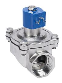
GC Valves potable water solenoid valve, 2-port (2-way), 2-position, N.C., 316 stainless steel body, 1-1/2in female NPT inlet(s), 1-1/2in female NPT outlet(s), Cv=13, 24 VDC operating voltage, 10W, NSF/ANSI/CAN 61.
