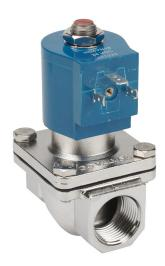
GC Valves potable water solenoid valve, 2-port (2-way), 2-position, N.C., 316 stainless steel body, 3/4in female NPT inlet(s), 3/4in female NPT outlet(s), Cv=6.7, 24 VDC operating voltage, 10W, NSF/ANSI/CAN 61.
