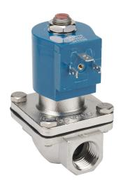
GC Valves potable water solenoid valve, 2-port (2-way), 2-position, N.C., 316 stainless steel body, 1/2in female NPT inlet(s), 1/2in female NPT outlet(s), Cv=4.3, 24 VDC operating voltage, 10W, NSF/ANSI/CAN 61.
