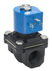
GC Valves potable water solenoid valve, 2-port (2-way), 2-position, N.C., Nylon 6 body, 3/4in female NPT inlet(s), 3/4in female NPT outlet(s), Cv=6.7, 120/110 VAC operating voltage, 8W.
