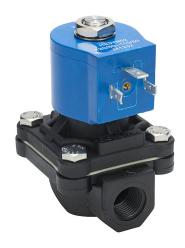
GC Valves potable water solenoid valve, 2-port (2-way), 2-position, N.C., Nylon 6 body, 3/8in female NPT inlet(s), 3/8in female NPT outlet(s), Cv=4.3, 120/110 VAC operating voltage, 8W.
