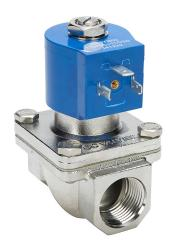
GC Valves potable water solenoid valve, 2-port (2-way), 2-position, N.C., 316 stainless steel body, 3/4in female NPT inlet(s), 3/4in female NPT outlet(s), Cv=6.7, 120/110 VAC operating voltage, 8W.
