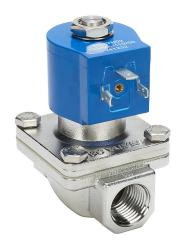
GC Valves potable water solenoid valve, 2-port (2-way), 2-position, N.C., 316 stainless steel body, 1/2in female NPT inlet(s), 1/2in female NPT outlet(s), Cv=4.3, 120/110 VAC operating voltage, 8W.
