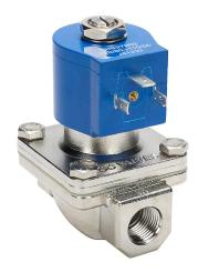
GC Valves potable water solenoid valve, 2-port (2-way), 2-position, N.C., 316 stainless steel body, 3/8in female NPT inlet(s), 3/8in female NPT outlet(s), Cv=4.3, 120/110 VAC operating voltage, 8W.
