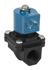
GC Valves potable water solenoid valve, 2-port (2-way), 2-position, N.C., Nylon 6 body, 3/4in female NPT inlet(s), 3/4in female NPT outlet(s), Cv=6.7, 120/110 VAC operating voltage, 8W, NSF/ANSI/CAN 61.
