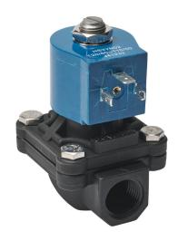
GC Valves potable water solenoid valve, 2-port (2-way), 2-position, N.C., Nylon 6 body, 1/2in female NPT inlet(s), 1/2in female NPT outlet(s), Cv=4.3, 120/110 VAC operating voltage, 8W, NSF/ANSI/CAN 61.
